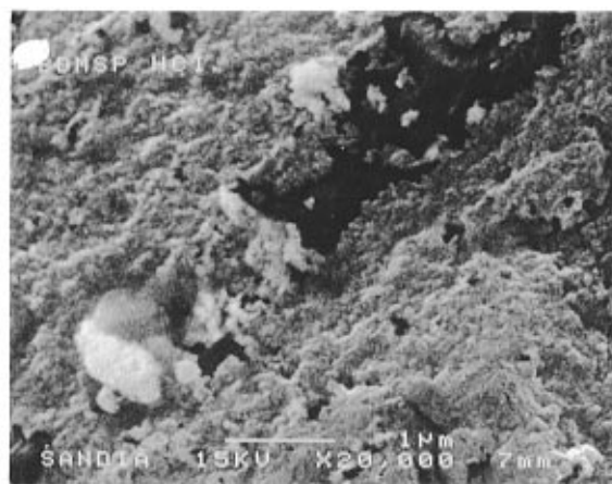
Figure 5. Scanning electron micrograph of phenylene-bridged polysiloxanes X-2-HCl and A-2-HCl .
